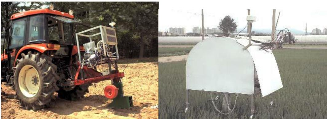
Figure 2. A soil organic matter content sensor (left), and a rice growth status sensor (right)
