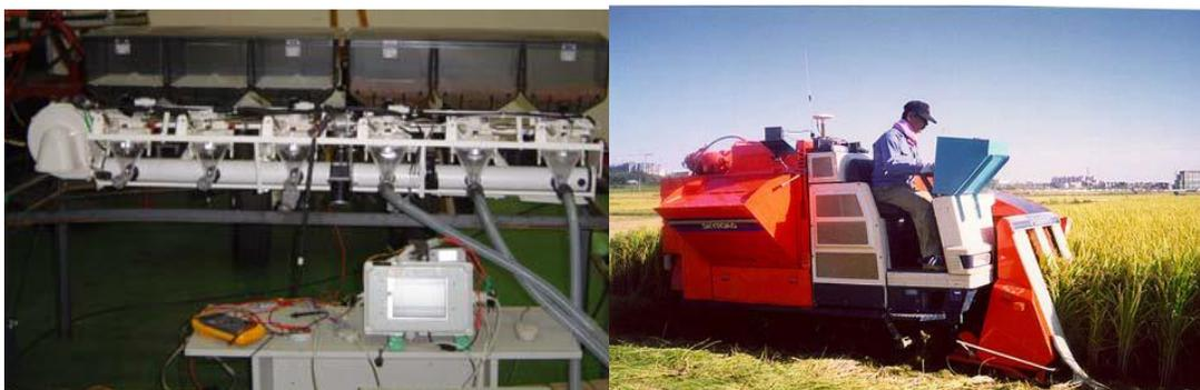
Figure 3. A variable rate granular fertilizer controller (left), and a rice yield monitoring system (right)
