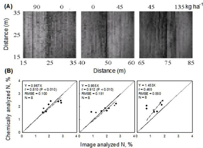
Fig. 3. (A) Maps of canopy N status of rice paddy obtained from three different regions of a rice field applied with different rates of N fertilizer, taken with a simplified imaging system unit mounted on a mobile lifter. (B) Validation of the relationships between the chemically analyzed and the image analyzed N (%) values from three different regions of a rice field applied with different rates of N fertilizer. (adapted from Lee *et al.*, 2008)
