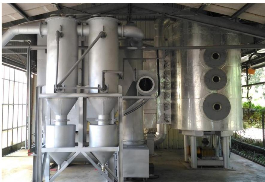
Fig. 1. 100 kg/hr (feeding rate) multiple hearth furnace with a continuous feeding system for mass production of biochar<sup>32</sup>
