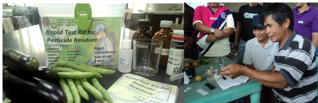
Fig.1. Rapid test kit (RTK) for the detection of organophosphate and carbamate residues on selected vegetables developed at the National Crop Protection Center, University of the Philippines Los Banos and farmer trying to use the RTK.
