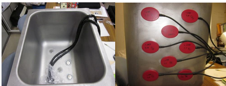
Fig. 3. Photographs of ultrasound chamber for treatment of agricultural crops
