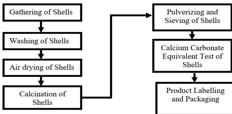
Figure 1. Standardized procedure for production of lime from shellfishes.
